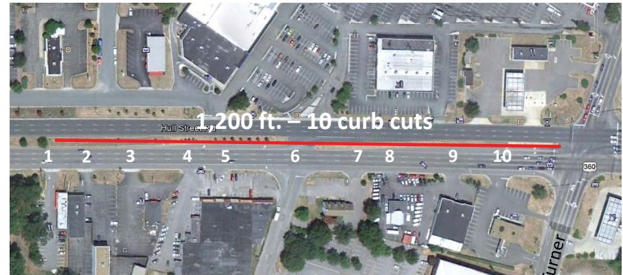
Figure 3.11: Spacing of curb cuts at this location is too close
